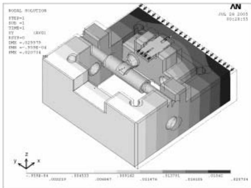
(b) Thermal deformation distribution in axial direction of case 2
