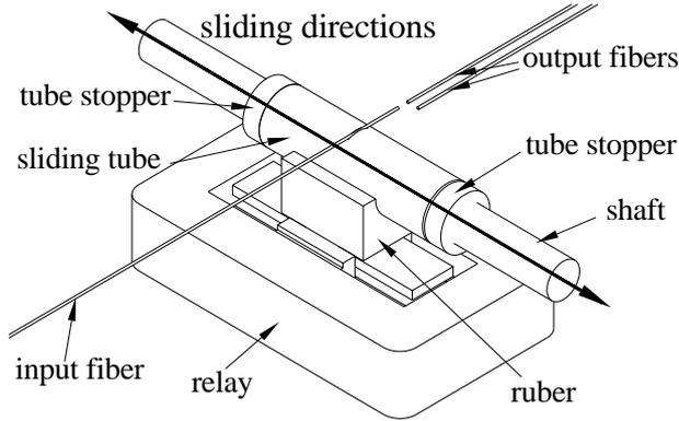
Fig. 1 The switching mechanism of the optical switch
