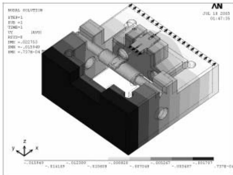
(a) Thermal deformation distribution in axial direction of case 1
