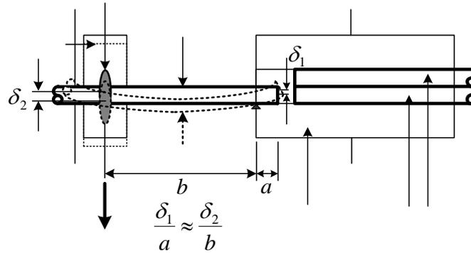
Fig. 3 Principle of the fiber stopper pivot design
