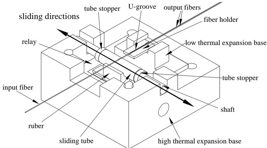
Fig. 2 The configuration of the optical switch
