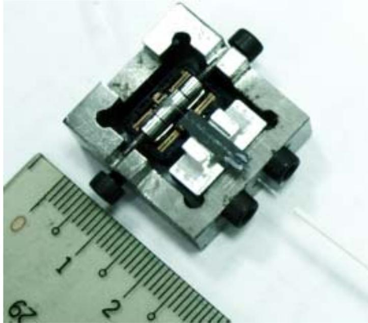
Fig. 6 Photo of the developed 1x2 optical switch
